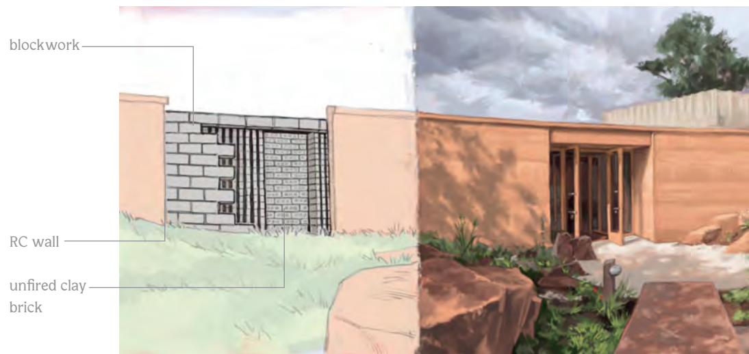
Above: Cutaway drawing of the natural air conditioning at The Weston
